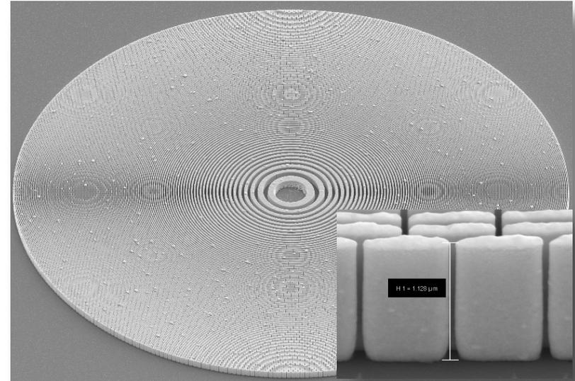
SEM-image of the FZP. Inset shows the thickness of the zones tilted at 45 degrees.
